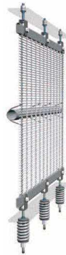
Mounting solution for wire mesh facades.
